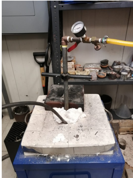
Figure 3. Assembly of the infiltration device and injection nozzle for the manufacture of metal foams.
