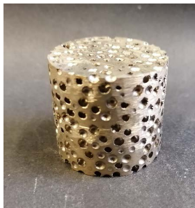
Figure 4. Syntactic Cu_{20}Sn metal foam using iron hollow spheres.
