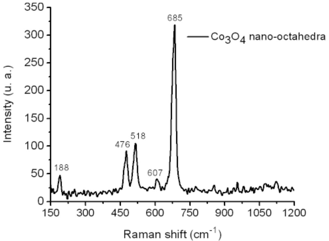
Fig. 5. Raman spectrum of  $\text{Co}_3\text{O}_4$  nano-octahedral.
