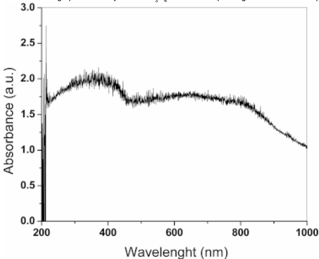
**Fig. 4.** UV-visible electronic absorption spectrum of  $\text{Co}_3\text{O}_4$  Nps.
