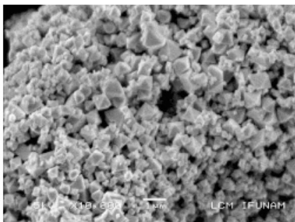
**Fig. 2.** SEM micrograph of  $\text{Co}_3\text{O}_4$  nanoparticles. Note the spinel octahedral morphology.
