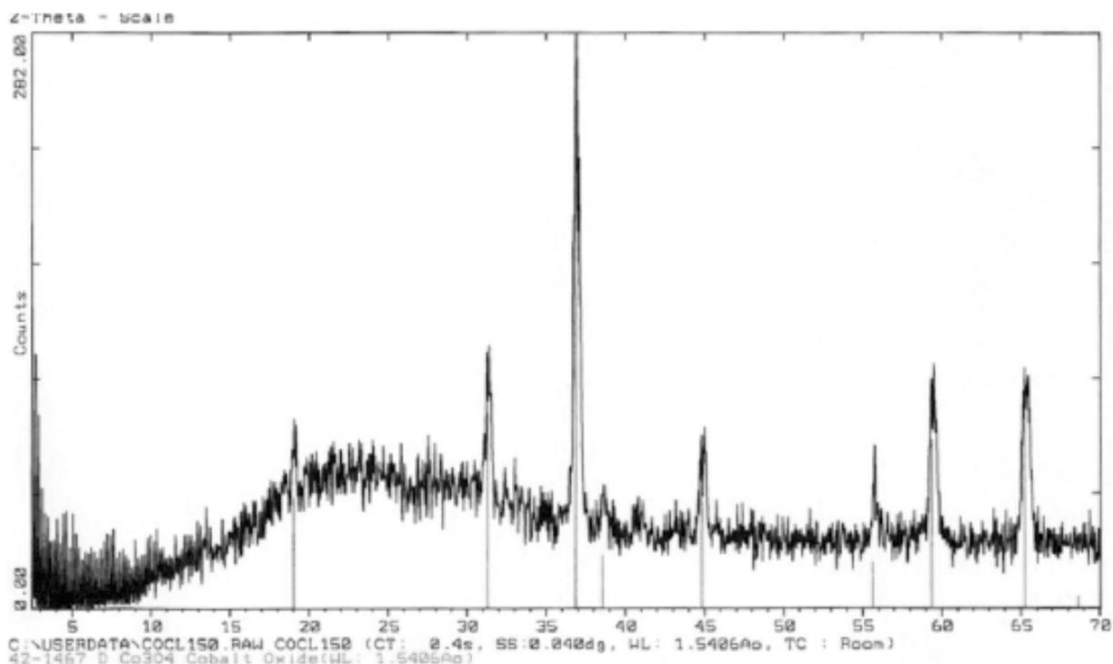
**Fig. 1.** XRD pattern of  $\text{Co}_3\text{O}_4$  nanoparticles. All peaks can be indexed to  $\text{Co}_3\text{O}_4$  cobaltite, with structure given by JCPDS No.421467.
