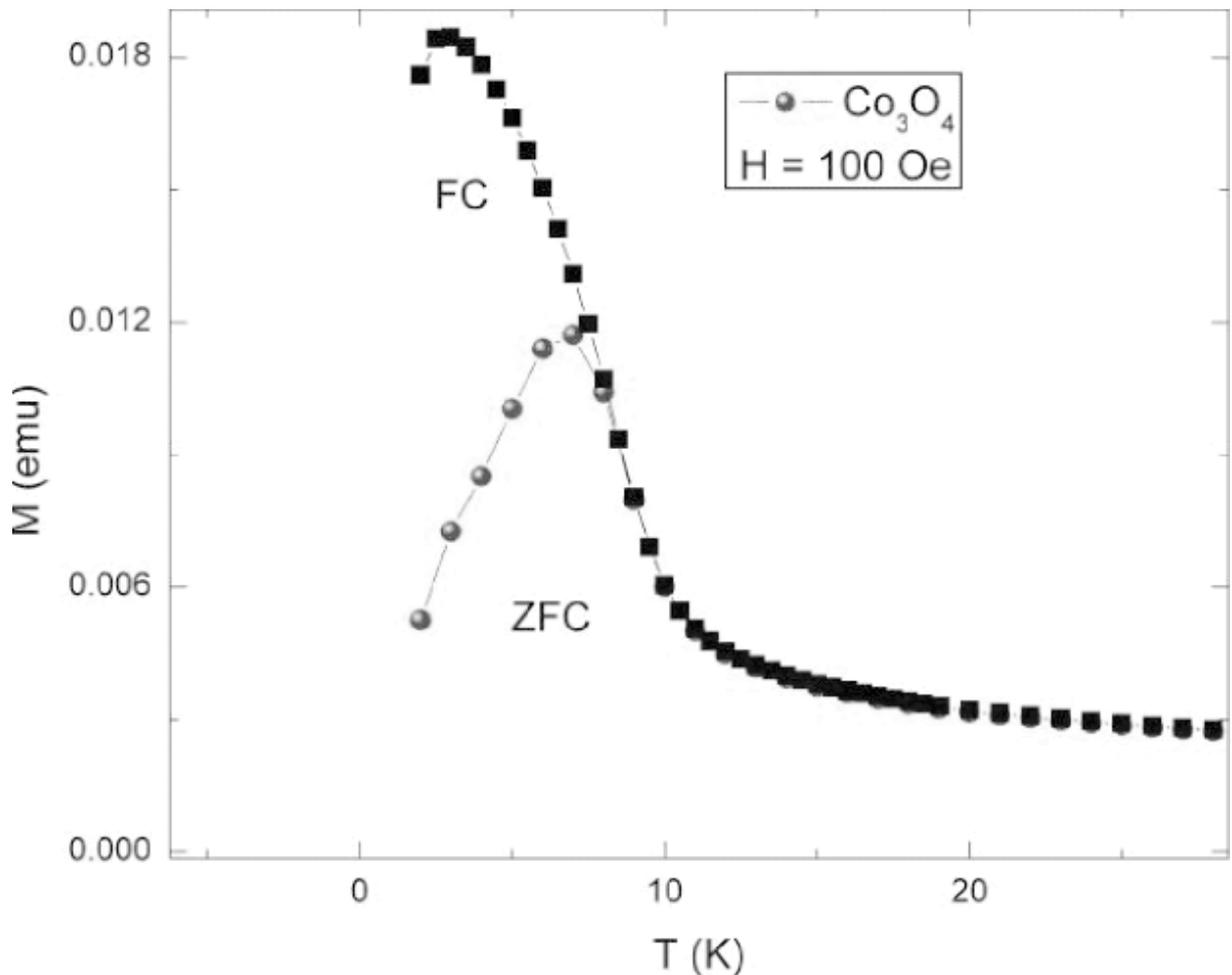
Fig. 6. Temperature dependence of FC and ZFC magnetization for  $\text{Co}_3\text{O}_4$  nanoparticles.
