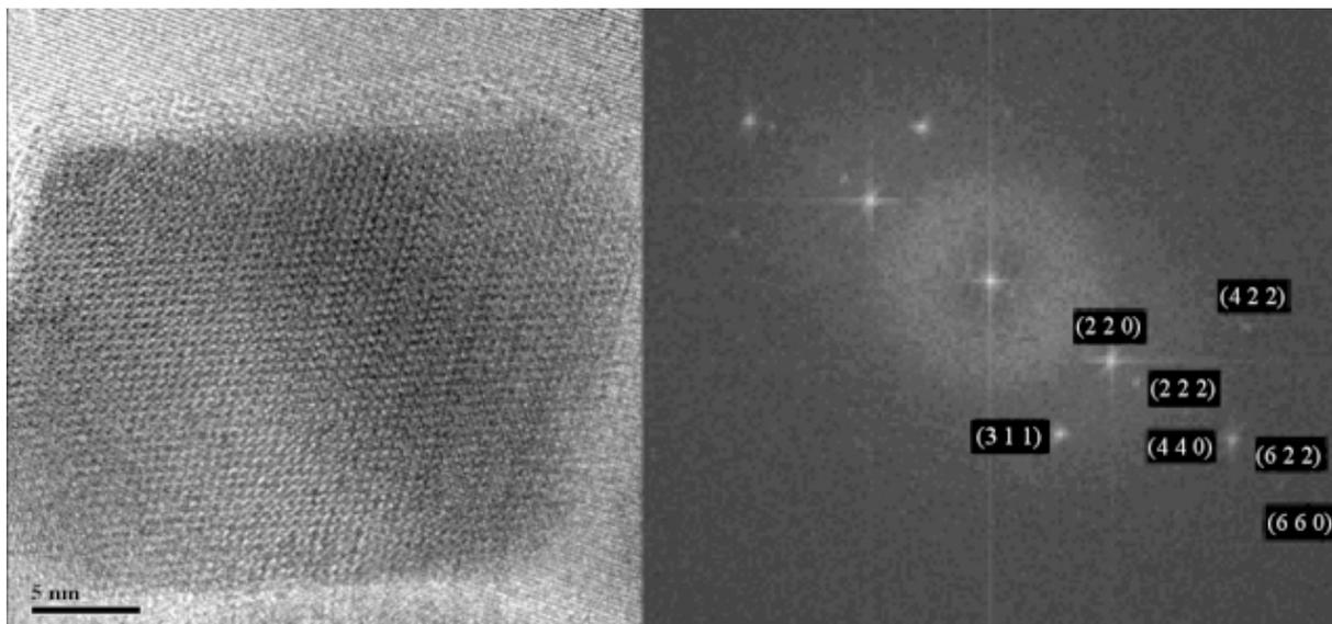
**Fig. 3.** HR-TEM micrograph of nanocrystalline  $\text{Co}_3\text{O}_4$  and its corresponding electron diffraction pattern.
