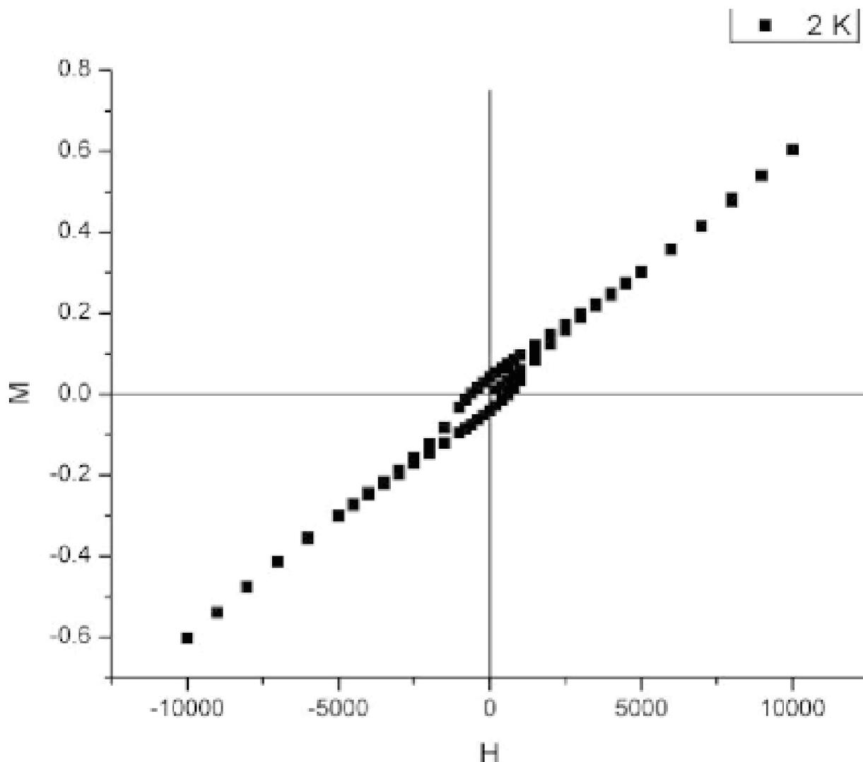
Fig. 7. Hysteresis loop obtained at 2K.
